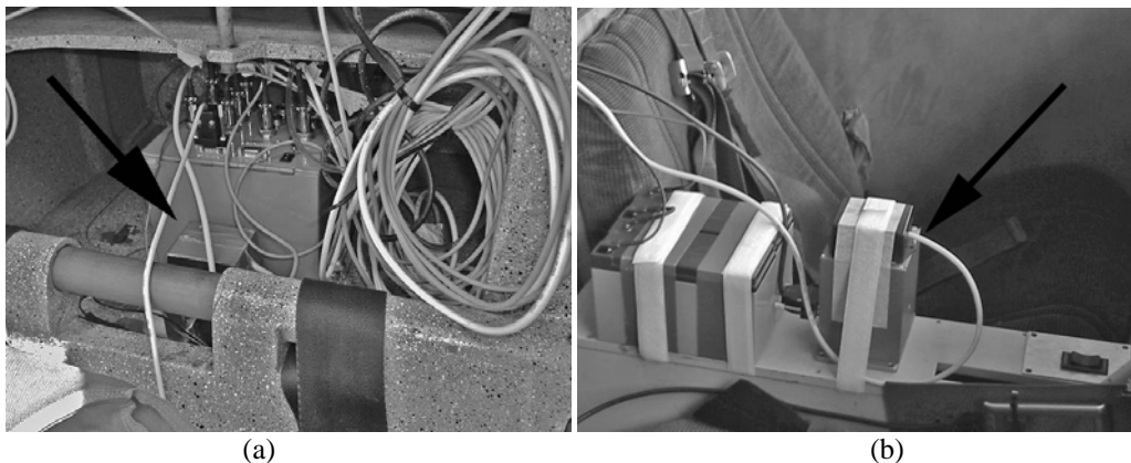
Figure 3. Puchaz (a) and Curumim (b) inertial platform and three axial accelerometer installation
